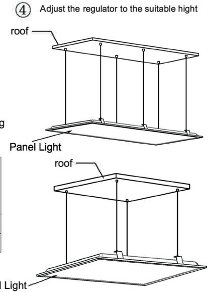
If the installation surface is too narrow, we suggest making the two fixing parts near to each other, please refer to drawing below.
