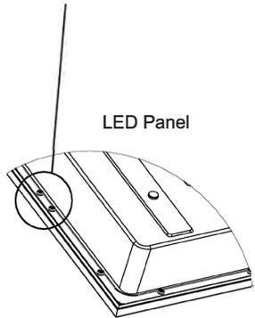
② Fix the hanging parts with M3\*8 screws
