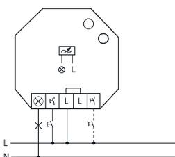
Control by pushbutton switches or light switches.
